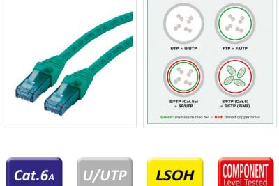
Patch cable for networking connections between devices. Prepared unshielded Twisted Pair cable with RJ-45 connectors on both ends. Durable due to moulded kink protection. Flexible cable, suitable for narrow bending. High quality plugs with gold plated contacts. Contact settings 1:1, in accordance with the EIA/TIA 568 standard. Construction: 4-pair stranded copper wire.
