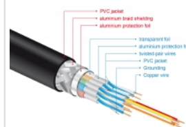
Triple shielding for lossless signal transfer
